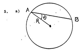
A straight line, frictionless track runs in a tunnel from point A to B through earth of constant density. What is the travel time as a function of  $\theta$  for a train propelled by gravity?
